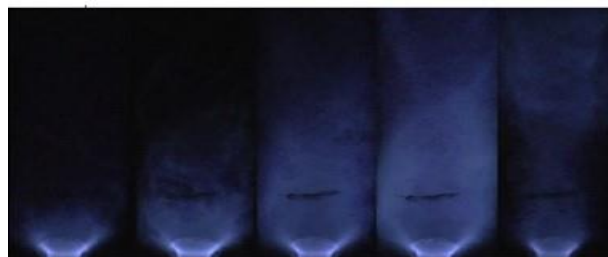
Figure 7: Pulsating flame. Progression of LBO seconds before final onset. S = 1.05 , \Phi = 0.525 . Frequency 10Hz.
